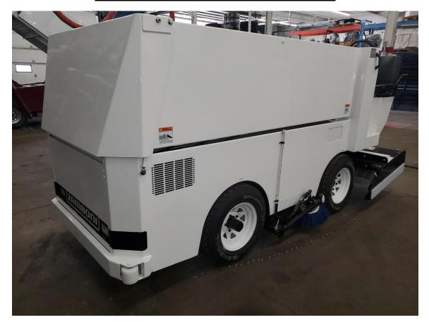
Zamboni resurfacer, model 445 refurbished with propane carburetion, built 2009
